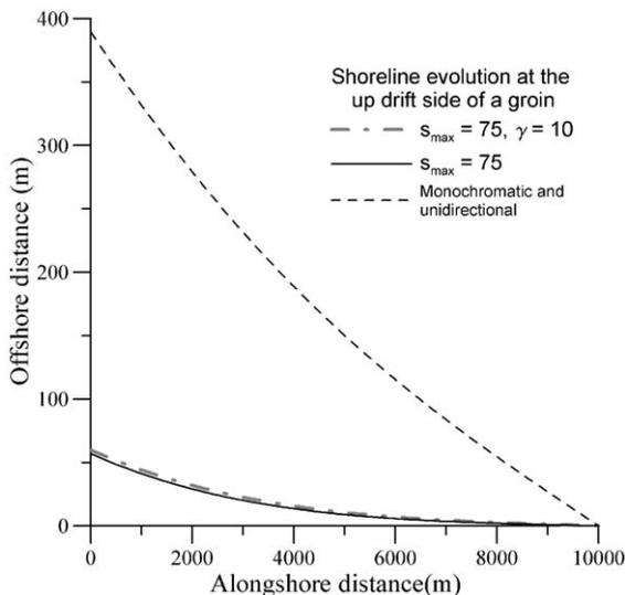
Fig. 2. Shoreline evolution at the up drift side of a groin for an initially straight beach. Two solutions for irregular swell forcing waves versus monochromatic and unidirectional forcing waves (adopted from Payo et al., 2003).
