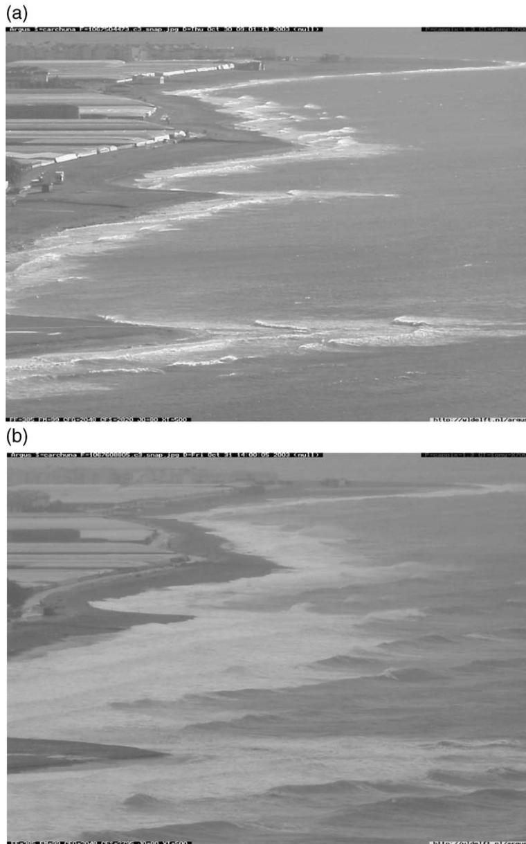
Fig. 1. Images from the ARGUS Station installed at Carchuna (SW wave incoming direction) under (a) mild wave conditions and (b) storm conditions.
