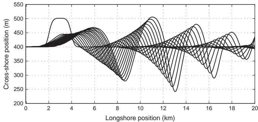
**Fig. 3.** Time evolution of the shoreline for the beach nourishment scenario and default offshore wave conditions. The shoreline is plotted every 6 months and the final line corresponds to the result after 8 years. Notice the exaggeration in the cross-shore axis.
