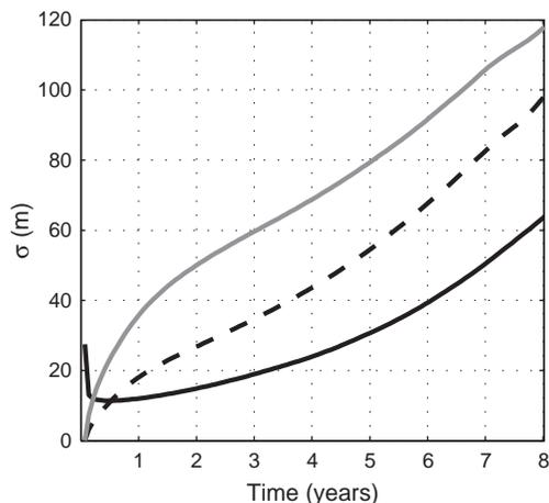
Fig. 6. Time evolution of the standard deviation of the shoreline using the default offshore wave conditions for the beach nourishment case (black solid line), the shoreface nourishment case (black dashed line) and the dredge pit case (grey solid line).
