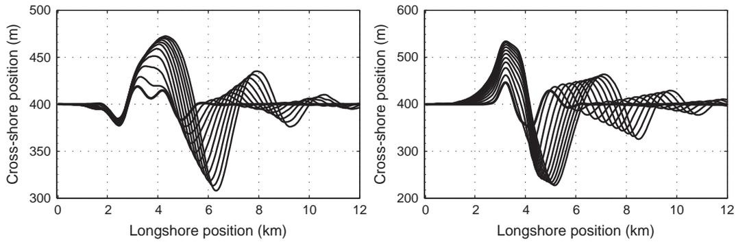
**Fig. 7.** Initial development of the shoreline for the shoreface nourishment scenario (left panel) and the borrow pit scenario (right panel) using the default offshore wave conditions. The shoreline is plotted every 3 months and the final line corresponds to the result after 2 years. Notice the exaggeration in the cross-shore axis.
