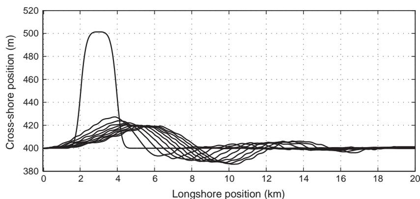
**Fig. 10.** Time evolution of the shoreline for the beach nourishment scenario with default wave height and period but weekly alternating wave angles of  $60^\circ$  and  $40^\circ$  (even contribution of unstable and stable conditions). The shoreline is plotted every 2 years and the final line corresponds to the result after 20 years. Notice the exaggeration in the cross-shore axis.
