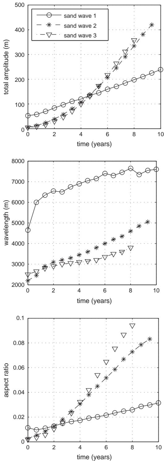
**Fig. 4.** The evolution of the total amplitude (crest to trough), the wavelength and the aspect ratio (total amplitude divided by wavelength) for the beach nourishment scenario and default wave conditions. The 3 lines represent the first to third sand waves of the sand wave train.
