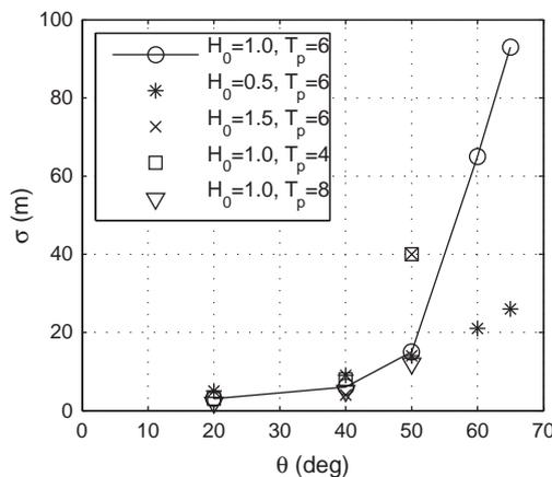
**Fig. 8.** Standard deviation of the final shoreline after 5 years for the shoreface nourishment case using different offshore wave conditions.
