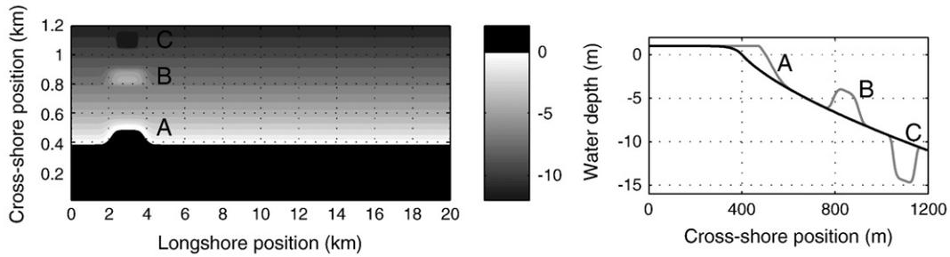
**Fig. 1.** Initial bathymetry (left panel) and cross-shore transect at  $y = 3$  km (right panel) showing the three possible nourishment scenarios: beach nourishment (A), shoreface nourishment (B), and borrow pit (C).
