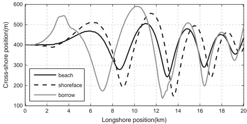
Fig. 5. Final shoreline after 8 years for the three nourishment scenarios and the default offshore wave conditions. Notice the exaggeration in the cross-shore axis.
