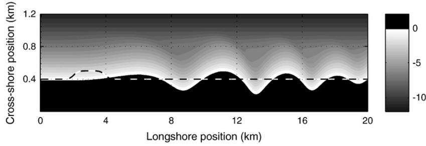
**Fig. 2.** Bathymetry after 8 years for the beach nourishment scenario and the default offshore wave conditions. The dotted line represents the initial shoreline with the beach nourishment. Notice the exaggeration in the cross-shore axis.
