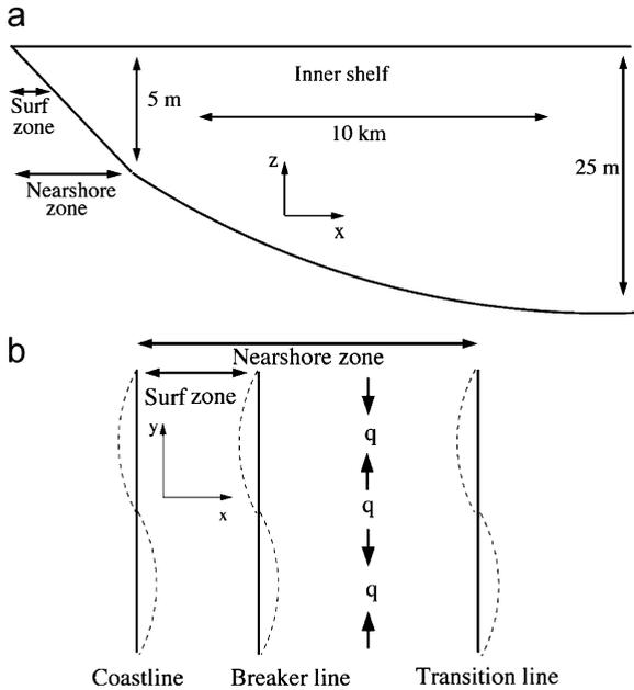
Fig. 2. (a) Side view of the geometry of the model; (b) top view of the model. The positions of the perturbed coastline, breaker line and transition line are indicated by dashed curves. It is assumed that the width of the nearshore zone is constant. The volumetric sediment flux in the alongshore direction is denoted by symbol  $q$  and occurs over the entire nearshore zone.
